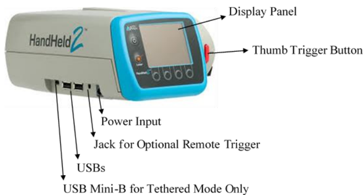
FIGURE 8. ASD FieldSpec HandHeld Spectroradiometer 2 (source: adapted from Malvern Panalytical).
